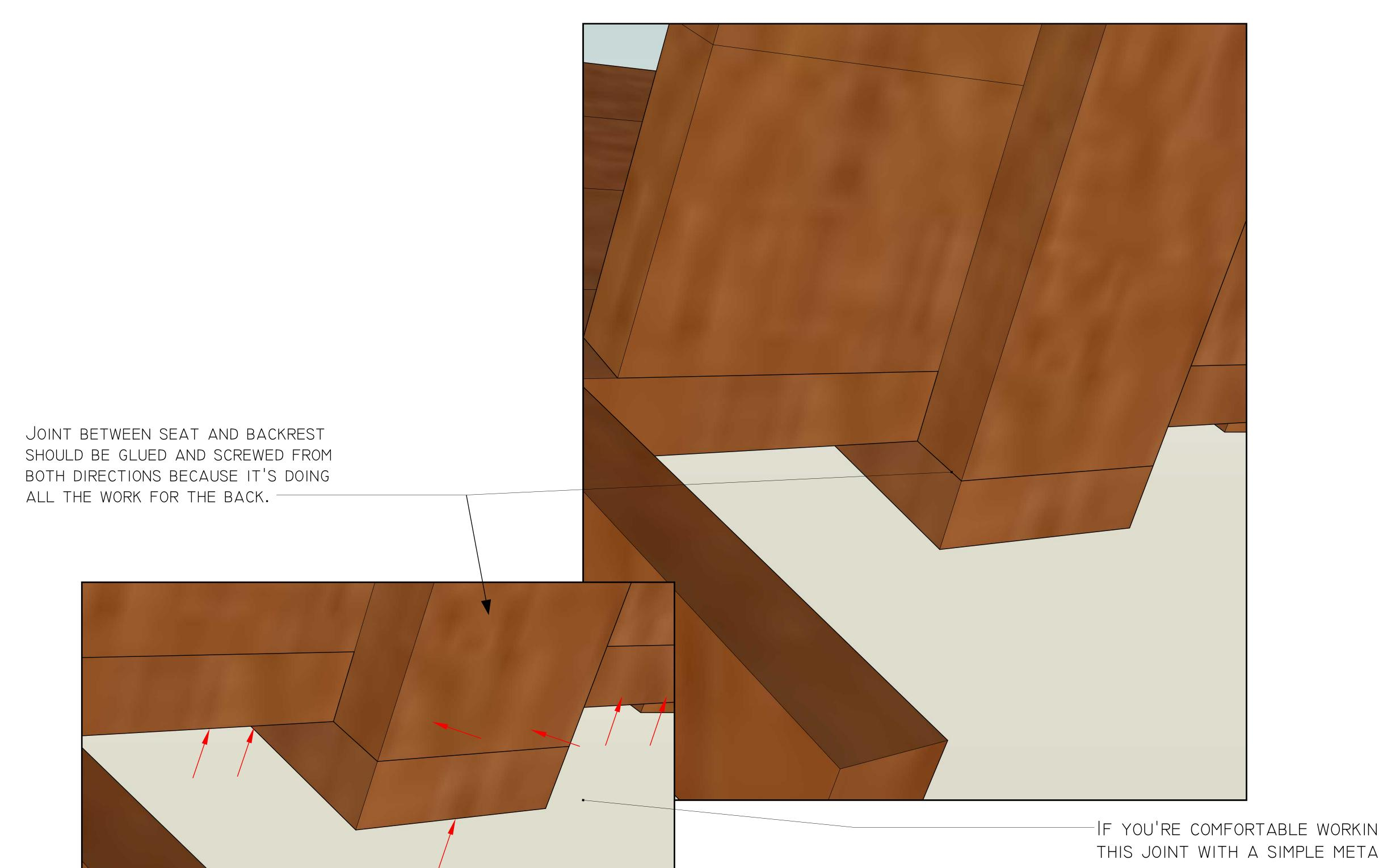
— IF YOU'RE COMFORTABLE WORKING WITH METAL YOU COULD REINFORCE THIS JOINT WITH A SIMPLE METAL BRACKET.
